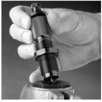
handle all the way and note the "feel" of the cam over in the linkage. With the handle all the way down, tighten the large die lock ring.
