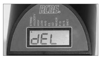
Figure 14 - Delete Current Velocity Data Point
