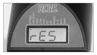
Figure 12 - Reset Display to Delete ALL Data
