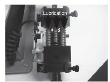
Photo 40: Lubricate Guide Rods and Spring Guide
