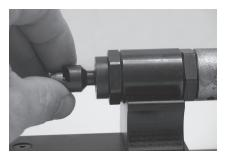
Photo 31: Installing Cutter Bushing and Cutter Head
