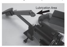
Photo 39: Handle Lever Lubrication Points
