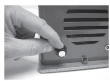
Photo 9: On/Off/Speed Control in Max RPM Position
