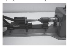
Photo 34: Slide Shell Holder Carrier Assembly to Cutter Shaft
