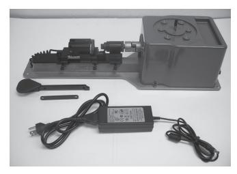
Universal Case Prep Center Handle Lever Assembly Handle Link DC Power Supply
