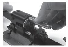
Photo 14: Removing Case from Universal Case Holder
